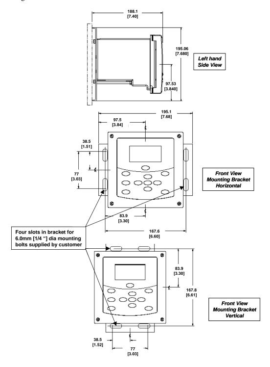
Figure 3-4 Wall Mounting Dimensions (not to scale)
